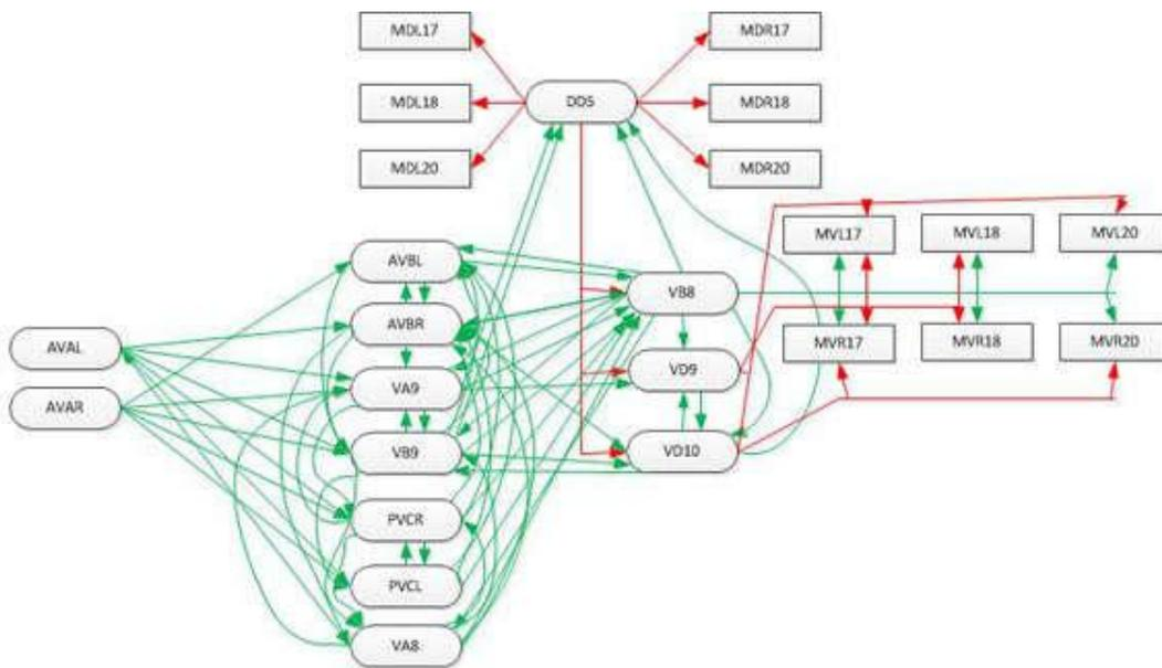
Currently the **connectome model** (modeled above) is being transferred to a Raspberry Pi and a self-contained Pi robot is being constructed. It is suggested that it might have practical application as some sort of mobile sensor - exploring its environment and reporting back results. Given its limited range of behaviors, it seems unlikely to be of practical value, but given more neurons this might change.
