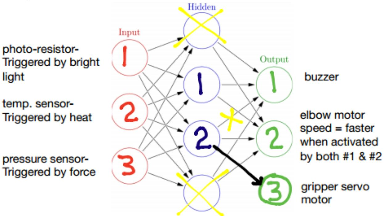
If temp and pressure sensor reach threshold, hidden layer #1 activates buzzer with a low tone (hot) and #2 activates gripper motor
