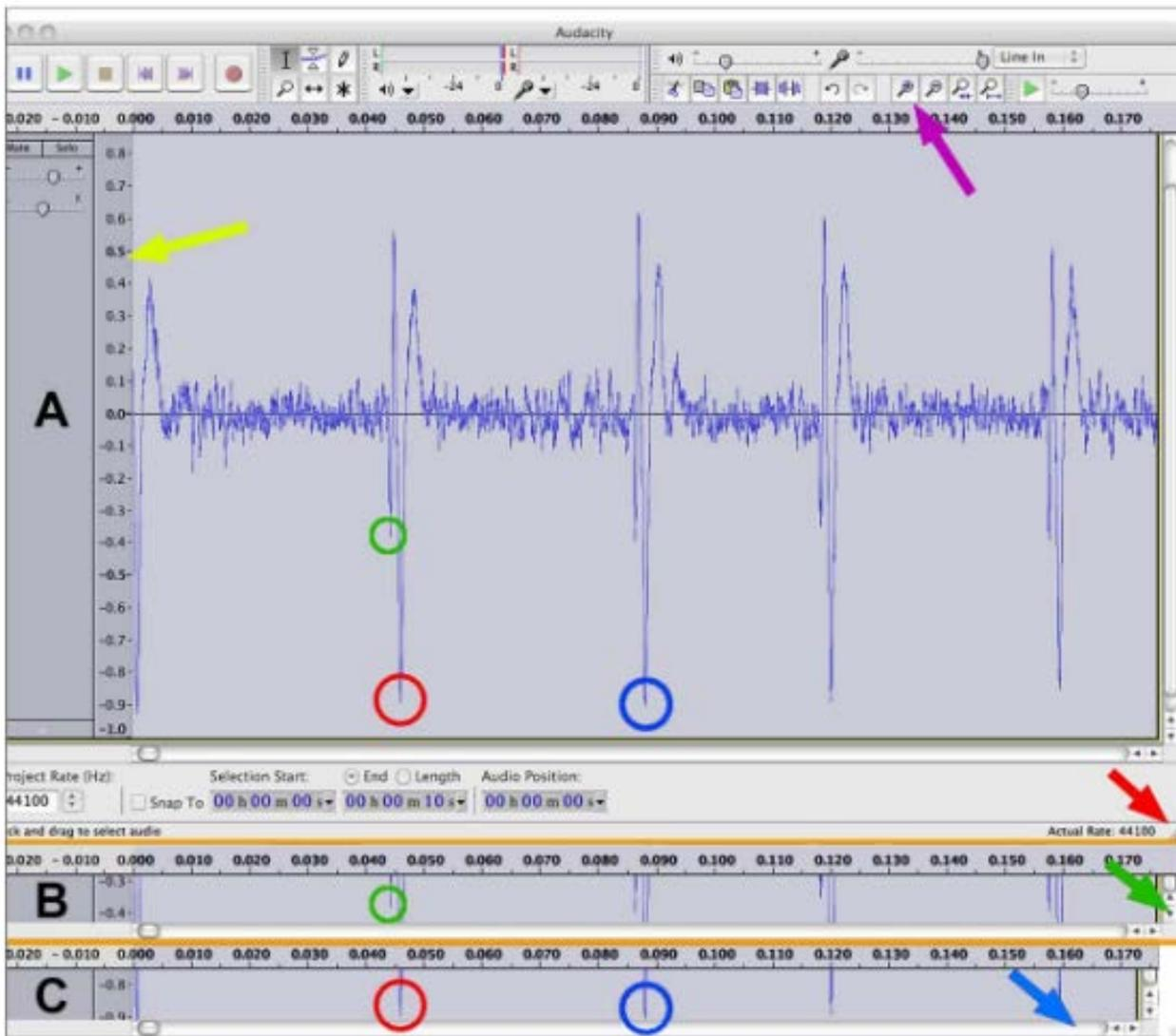
22. Isolate and amplify a five second section of recording using the above method. Ensure you have recorded the Amount of Amplification in **Table 2**.
